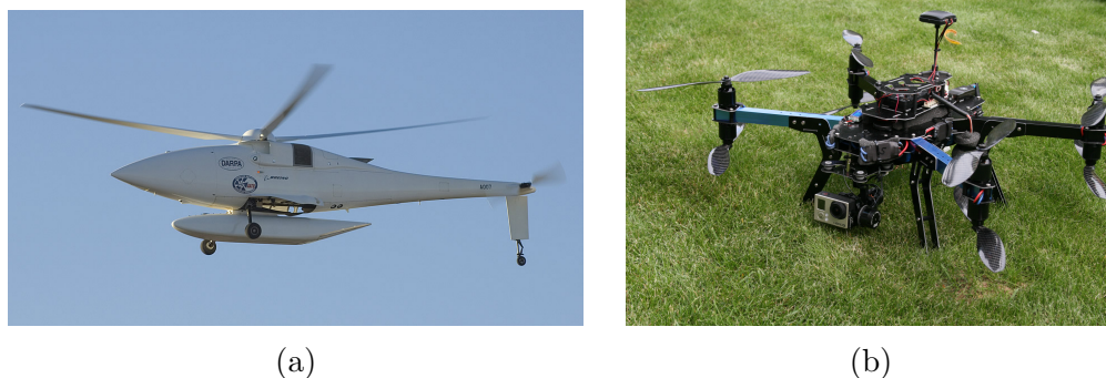
Figura 2.9: UAVs de ala rotativa: (a) boeing modelo A160T Hummingbird [Daily, 2016] y (b) 3DR modelo SX8-M [3DR, 2016].
